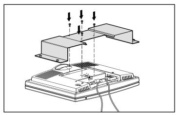
Figure 2-19. Attaching the fixed mounting bracket
